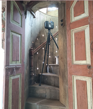
LiDAR Scanner used to document Havelis
